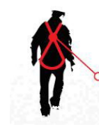
Fall FACTOR 2 anchor point located below the back anchor point of the harness
