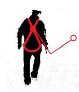
Fall FACTOR 1 anchor point located at the same level of the back anchor point of the harness
