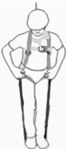
5. Stand onto the loop, so as to relieve the pressure of the harness webbing.
