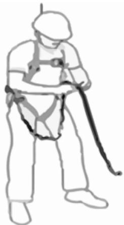
3. Connect the straps with each other making a loop with the help of buckle
