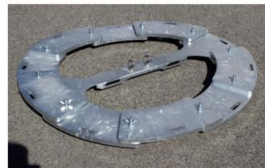
5. Connect the connector (EN 362:2004) of the fall arrester to the Orbyt anchorage rings and the other end to the harness anchorage point (EN 361:2002). Before use, the user must check that the Orbyt anchorage device is correctly installed. Make sure that it is positioned horizontally, firmly and stably supported. Disassembly of the device must be carried out in reverse order.
