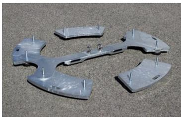
4. Fit the remaining 5 counterweights as shown in Fig. Secure the system with the wing nuts and tighten by hand.
